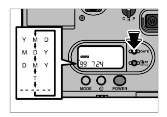
The date mode will alternate as shown in the diagram whenever the DATE Button is pressed.
